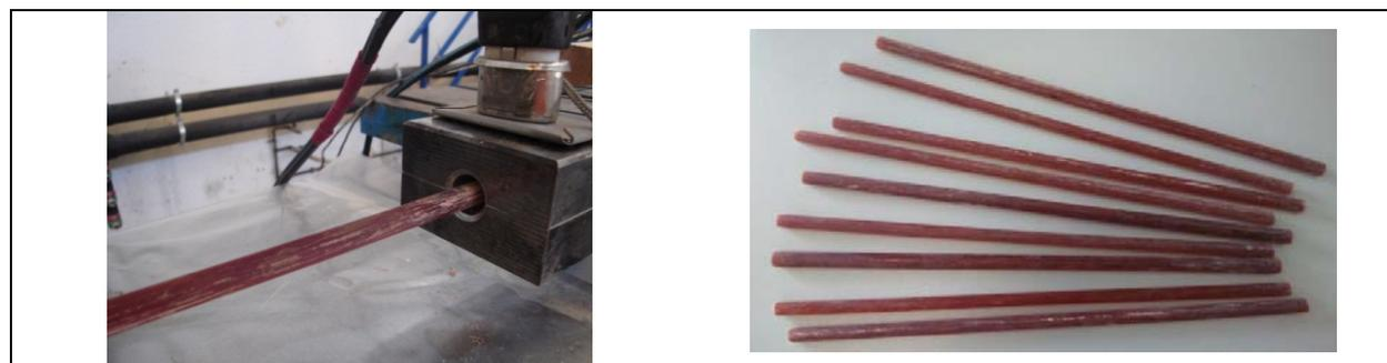
Figure 7. Optimised bioepoxy composite profiles obtained by pultrusion
