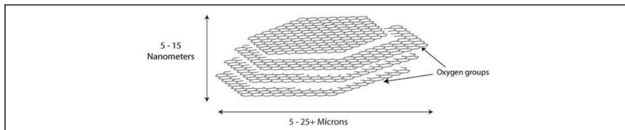
Figure 2. Typical scheme of configuration of graphene nanoplatelets.
