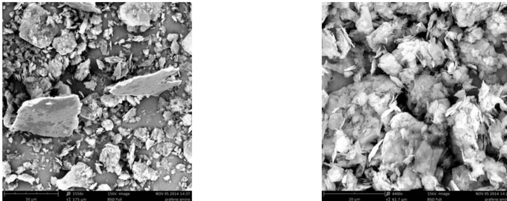
Figure 5. Graphene nanoplatelets modified with aminosilanes micrograph X1550, 4400.
