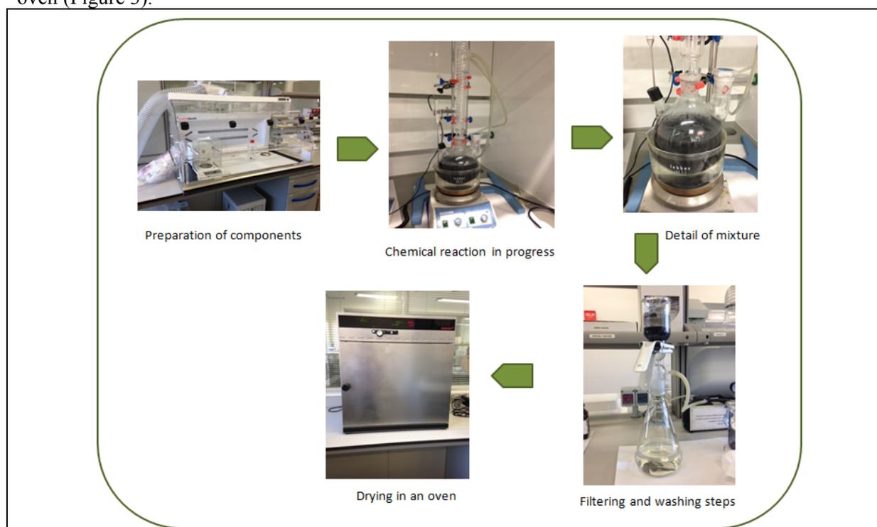
Figure 3. Phases of chemical modification reactions.
