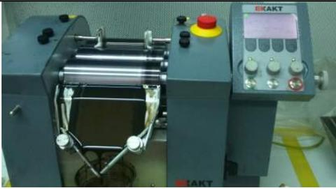
Figure 4. Dispersion of graphene by 3-roll mill at pilot plant
