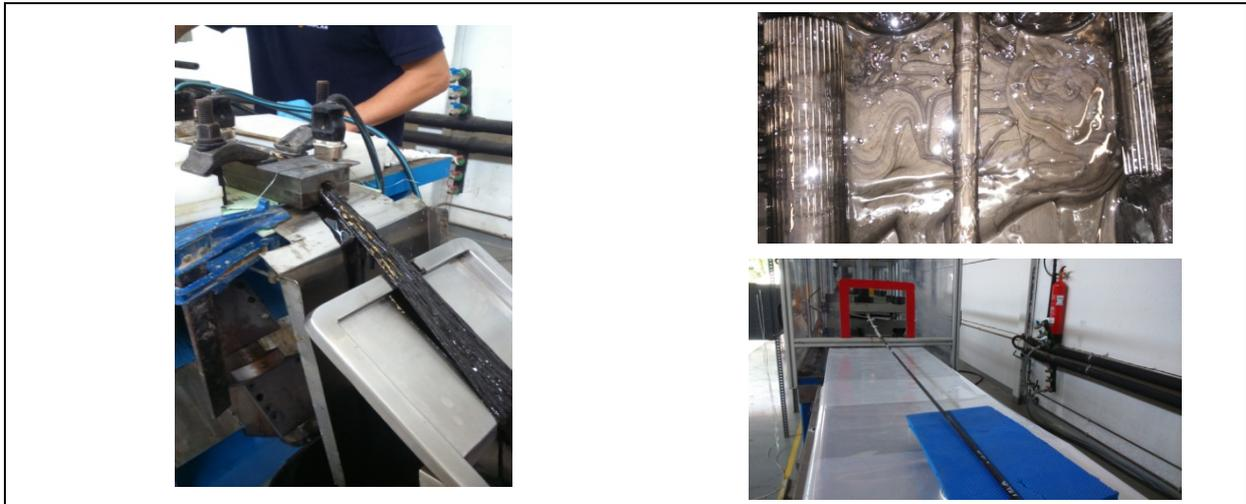
Figure 8. Pultrusion trials: Different steps of the manufacturing of bioepoxy and graphene composite profiles.
