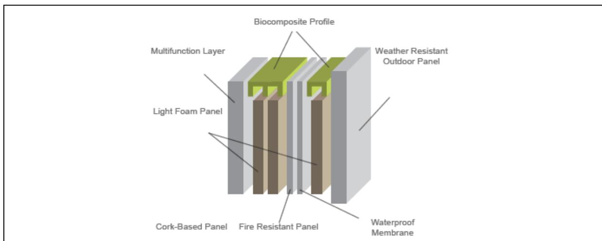
Figure 1. Assembled modular multi-layer envelope based on biocomposites in which is integrated developed biocomposite profile
