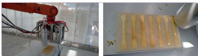
Fig. 6: MW antenna curing of tensile test pieces with a robot
